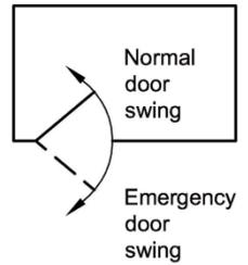
PIVOT CENTRES MUST BE IN LINE TO ENSURE SAFE AND CORRECT OPERATION
