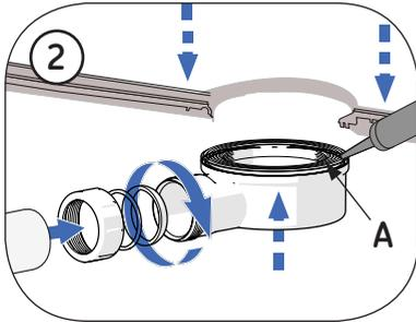
(2) Before fitting the waste, place the nut onto the waste pipe, followed by the backing ring and the seal. Insert waste pipe into the waste and tighten the nut. Check that the pipe connection is correctly assembled, sealed and watertight. Ensure that the seal (A) is positioned into the recessed section on the top of the waste body before connecting to the tray.
