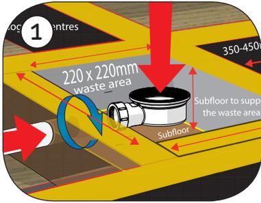
(1) As a “dry run”, first place the tray into the desired location and determine the position, the depth and the clearance required for the waste. Ensure there is sufficient support around the waste, see separate tray instructions.
